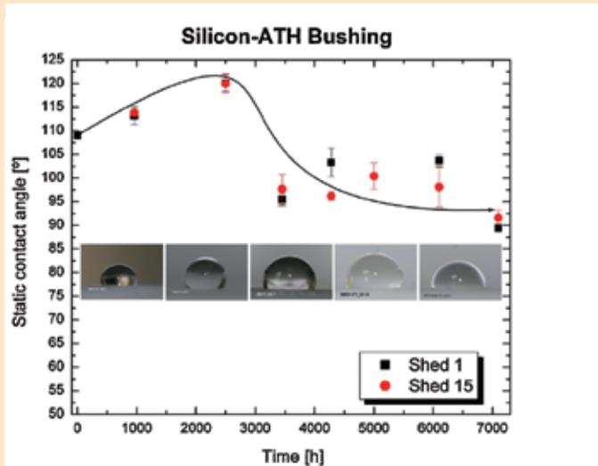
Figure 3. Static contact angle measurement vs. aging time for silicone-ATH bushing sample 4 tested in laboratory.
