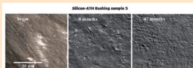
Figure 10. Microstructure images of non-ceramic housing of the bushing during different time of evaluation. Microstructure was analyzed by scanning electronic microscope using replica technique.
