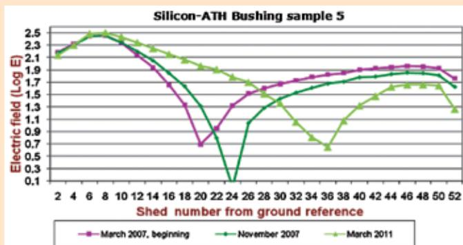
Figure 12. Electric field distribution along the non-ceramic bushing connected to the line.
