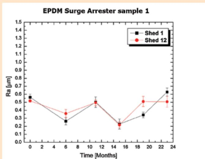
Figure 6. Surface roughness  $R_a$ , as a function of service time for EPDM-ATH arrestersample 1 installed in field.
