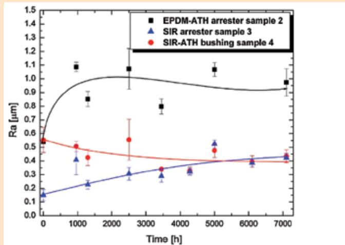
Figure 5. Surface roughness Ra, as a function of aging time for different polymer insulating materials tested in laboratory. Data of roughness correspond to the upper shed.
