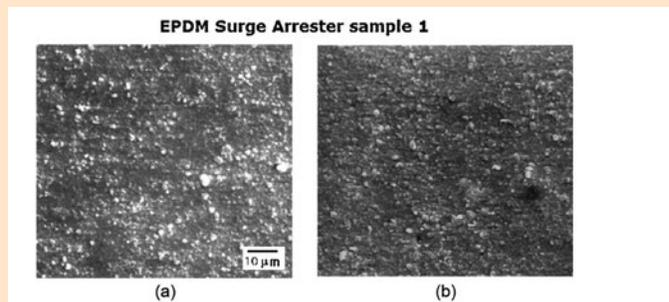
Figure 9. Replica surface microstructures of EPDM-ATH arrester sample 1 installed in field having 12 months of service.
