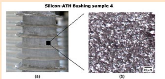
Figure 11. (a) Image showing the point on the sample where replica was taken. (b) Sheath surface microstructure of SiR-ATH housing material sample 4 taken by replica technique.
