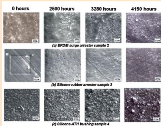
Figure 8. Surface microstructures obtained by replica technique for samples 2-4 at different aging test time.
