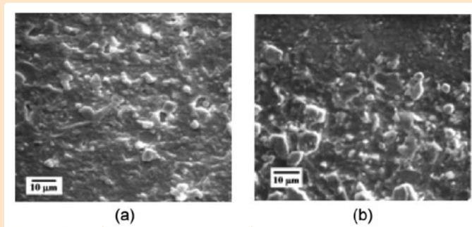
Figure 7. Surface microstructure of polymeric housing material: (a) direct observation and (b) replica technique.
