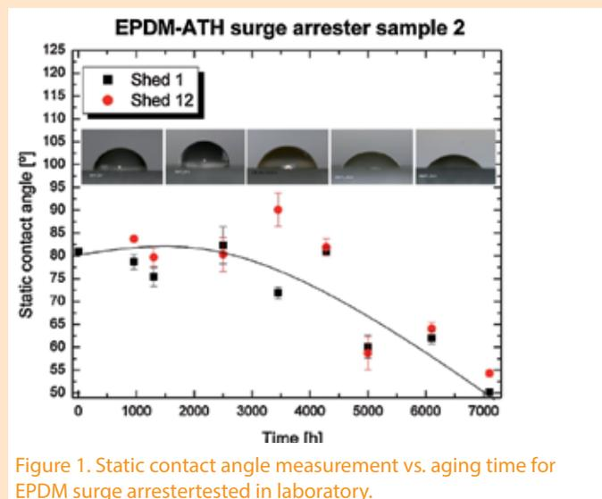
Figure 1. Static contact angle measurement vs. aging time for EPDM surge arrester tested in laboratory.
