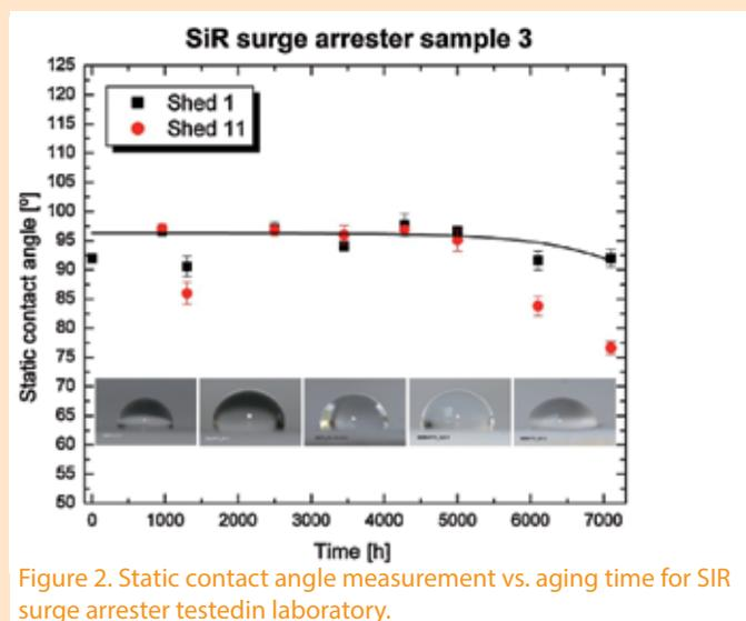
Figure 2. Static contact angle measurement vs. aging time for SiR surge arrester tested in laboratory.
