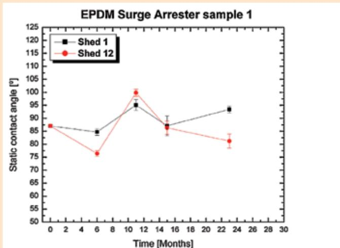
Figure 4. Static contact angle measurement vs. aging time for EPDM surge arrester tested in field.
